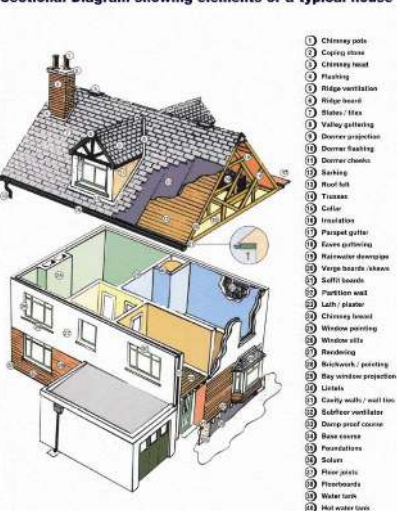
Sectional Diagram showing elements of a typical house
